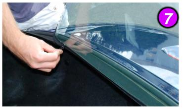
Insert the convertible top fabric into the rubber ring outdoors with a thin blade or a flat screwdriver:
