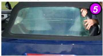
Mounting the new window: align the window zipper teeth (pink) with the first hood teeth (green) as shown in this picture, the silver teeth of the screen must be aligned with the very first teeth of the hood. The teeth of the end of the zipper of the new window are also silver, but these are the starting ones that are important.
